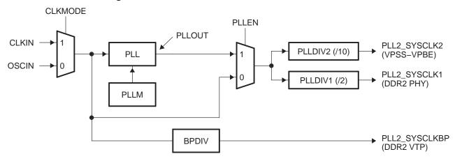
Figure 5-2. PLL2 Structure in the TMS320DM643x DMP
